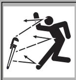
**⚠ DANGER** Moving tools will kill or injure. Shut off drill string power when anyone can be struck by moving or thrown tools. Never use pipe wrenches on drill string.
